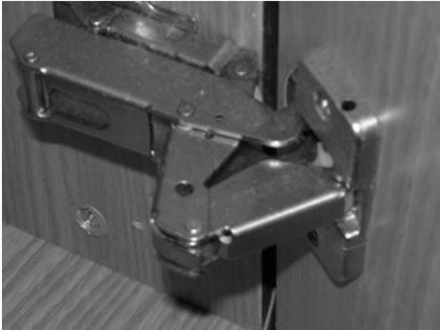
Figure 1: The curve scribing mechanism as a door hinge
